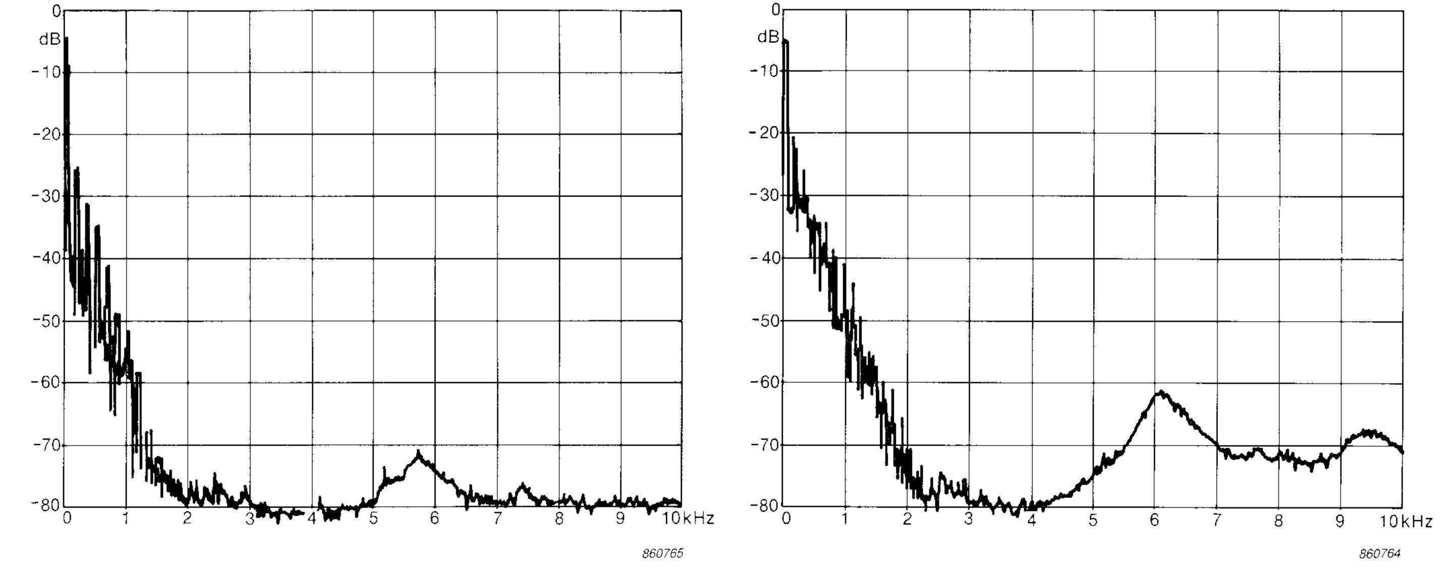
Fig. 13. Loudspeaker spectrum with noise-like peak near 6 kHz due to barely audible loose particle in gap (test tone 80 Hz)
