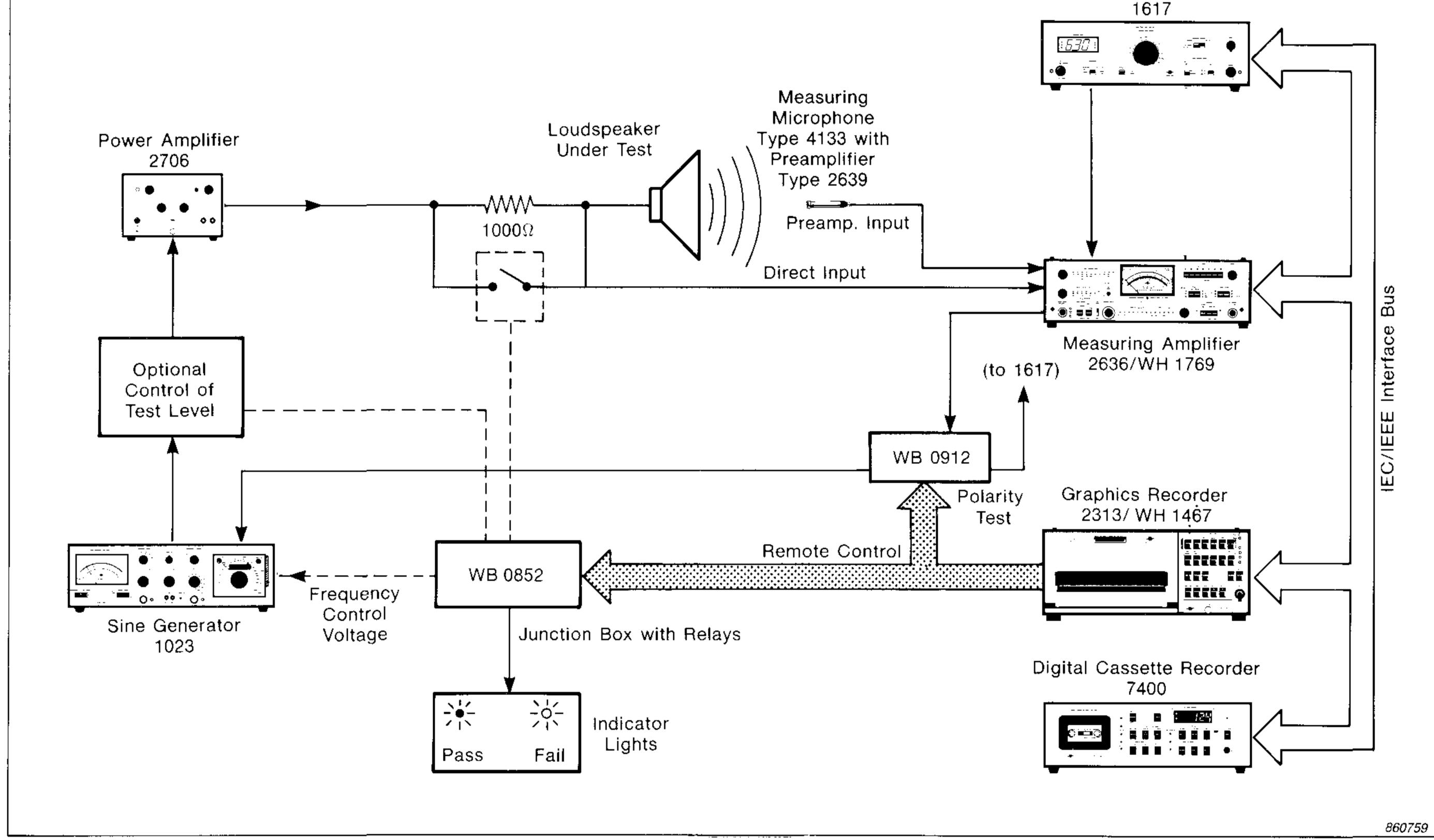
Fig. 26. Block diagram of automated loudspeaker test system
