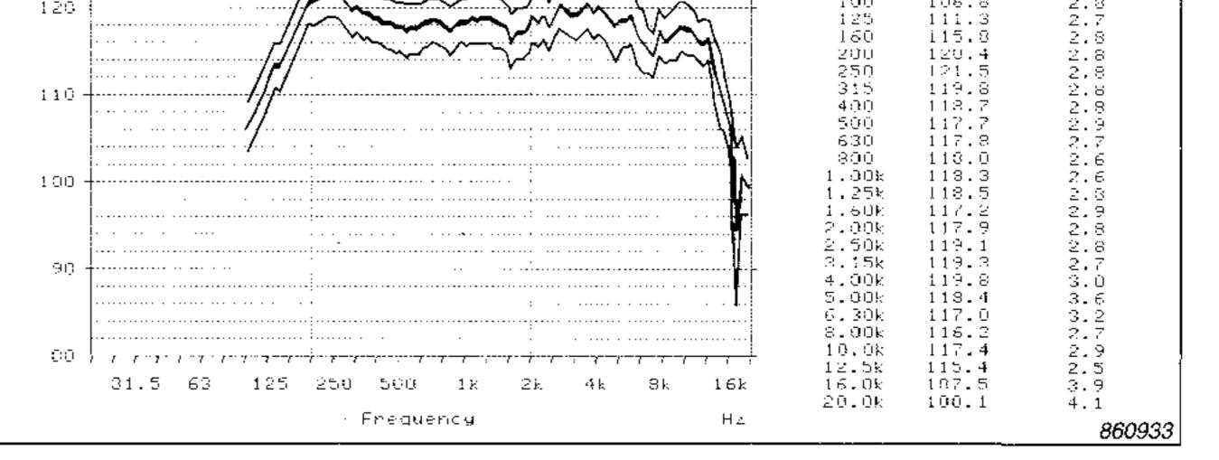
Fig. 23. Same speaker as Fig. 22. 3<sup>rd</sup> harmonic distortion 2% at 400 Hz
